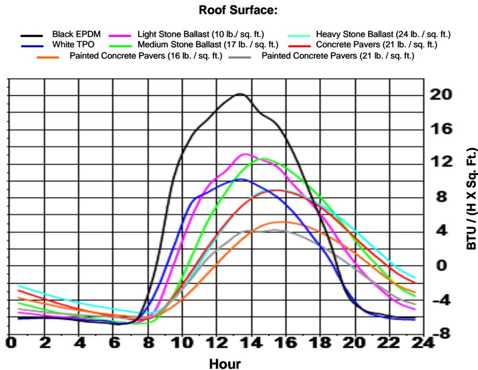
**Figure 1: Heat Flux through Roof by Hour**
