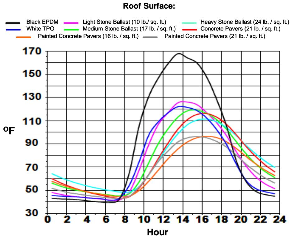
**Figure 2: Roof Membrane Temperature by Hour**
