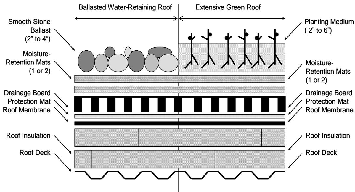
**Figure 3: Water-Retention Using Moisture Retention Mat(s)**
