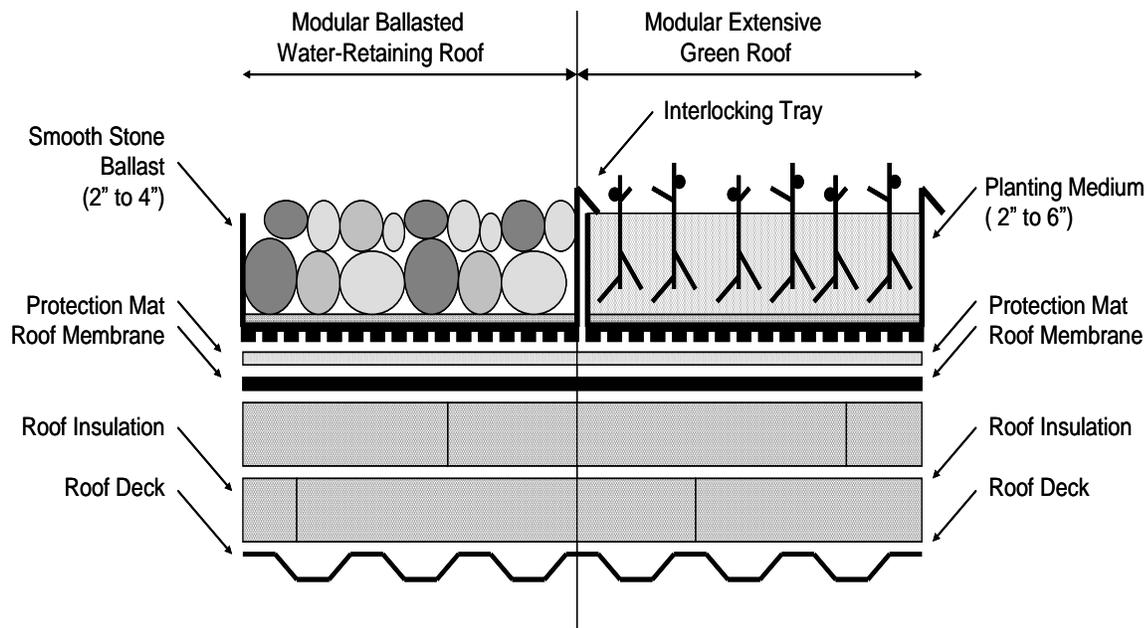
**Figure 4: Water-Retention Using Modular Trays**
